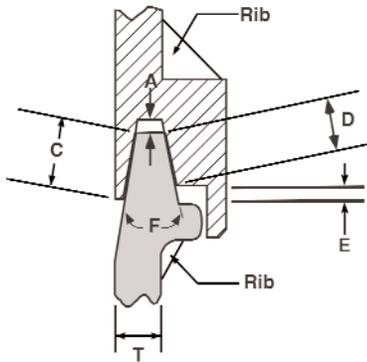
Figure 6. Tongue and Groove Joint with External Skirt
