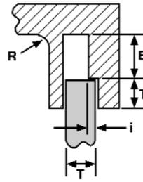
Figure 4. Flanged Shear Joint Design
