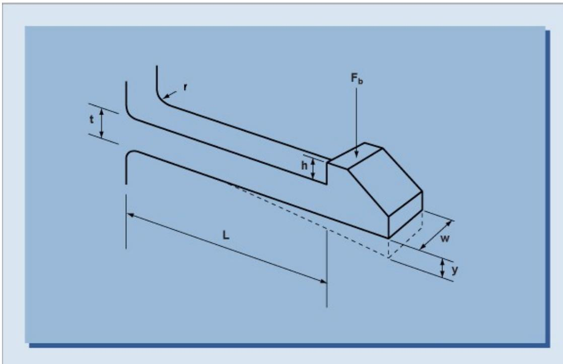
The maximum allowable deflection  $y$  and deflection force  $F_b$  can be calculated with the following formulas if the maximum allowable strain level  $\epsilon$  of the material is known.
