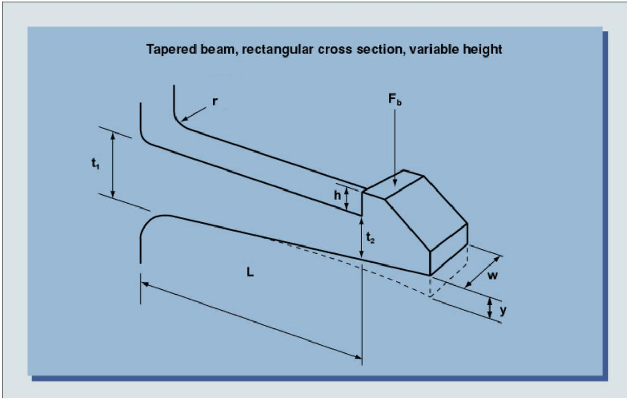
The following formulae can be used to calculate the maximum allowable deflection  $y$  and deflection force  $F_b$  for a tapered cantilever beam with a rectangular cross section. The height of the cross section decreases linearly from  $t_1$  to  $t_2$ , see figure above.
