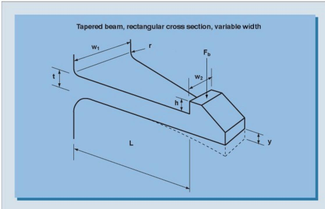
The following formulae can be used to calculate the maximum allowable deflection  $y$  and deflection force  $F_b$  for a tapered cantilever beam with a rectangular cross section. The width of the cross section decreases linearly from  $w_1$  to  $w_2$ , see figure above.
