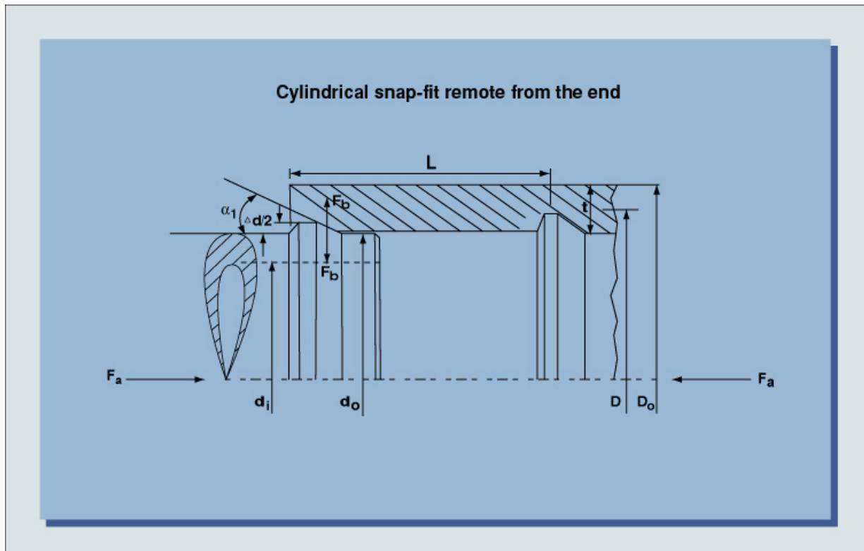
More material must be deformed if the snap fit is remote from the end, and the deflection force  $F_b$  and mating force  $F_a$  will be a factor 3.4 higher. The snap-fit is regarded as being remote if
