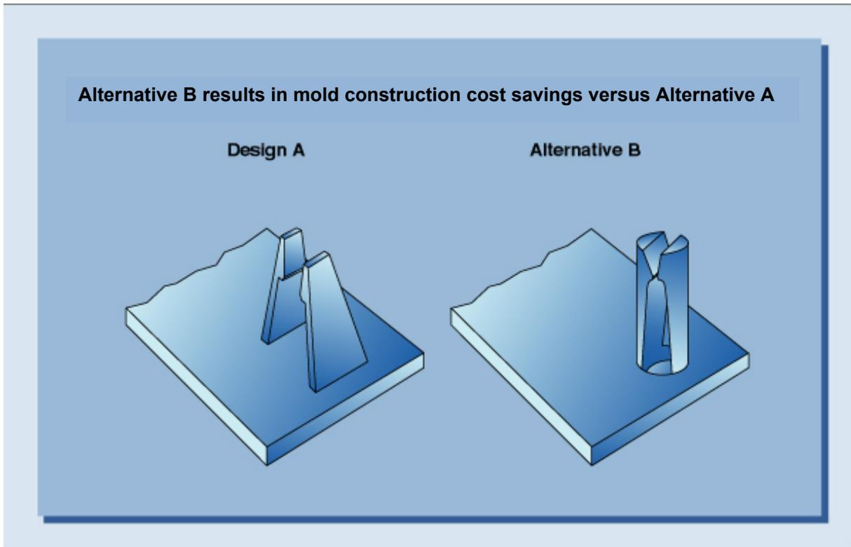
For design A, an expensive slide in the mold is required and the flat surfaces require expensive milling. No slide is required for alternative B and the cylindrical outside surface can simply be drilled.
